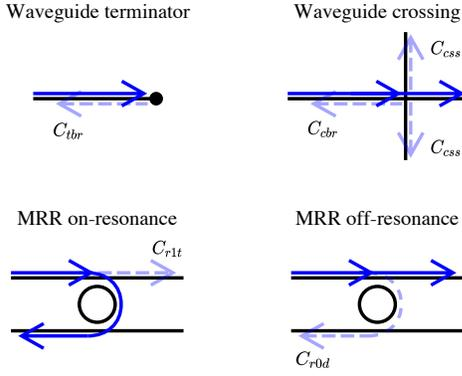
Figure 5. Noise sources in ONoCs: terminator back reflection ( $C_{tbr}$ ), crossing side spill ( $C_{css}$ ), crossing back reflection ( $C_{cbr}$ ), MRR on-resonance through ( $C_{r1t}$ ) and MRR off-resonance drop ( $C_{r0d}$ ). Full arrows are signal paths, dashed arrows are noise paths.
