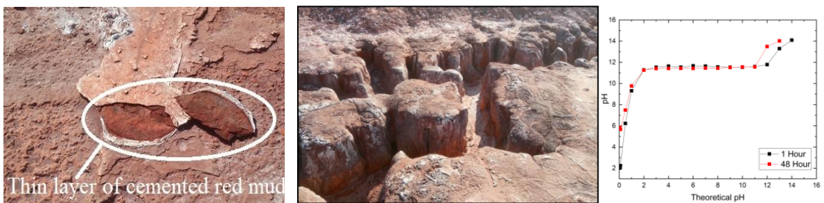
Buffer zone tests for the Bauxite residue
