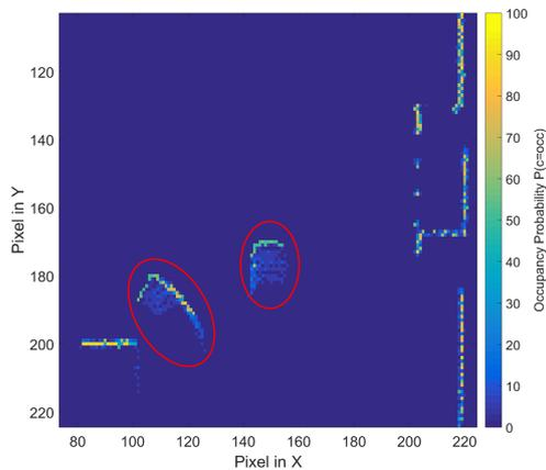
**Figure 4.8:** A snippet of the networks input visualizing spatio-temporal features of two moving robots with different shapes (red ellipses).
