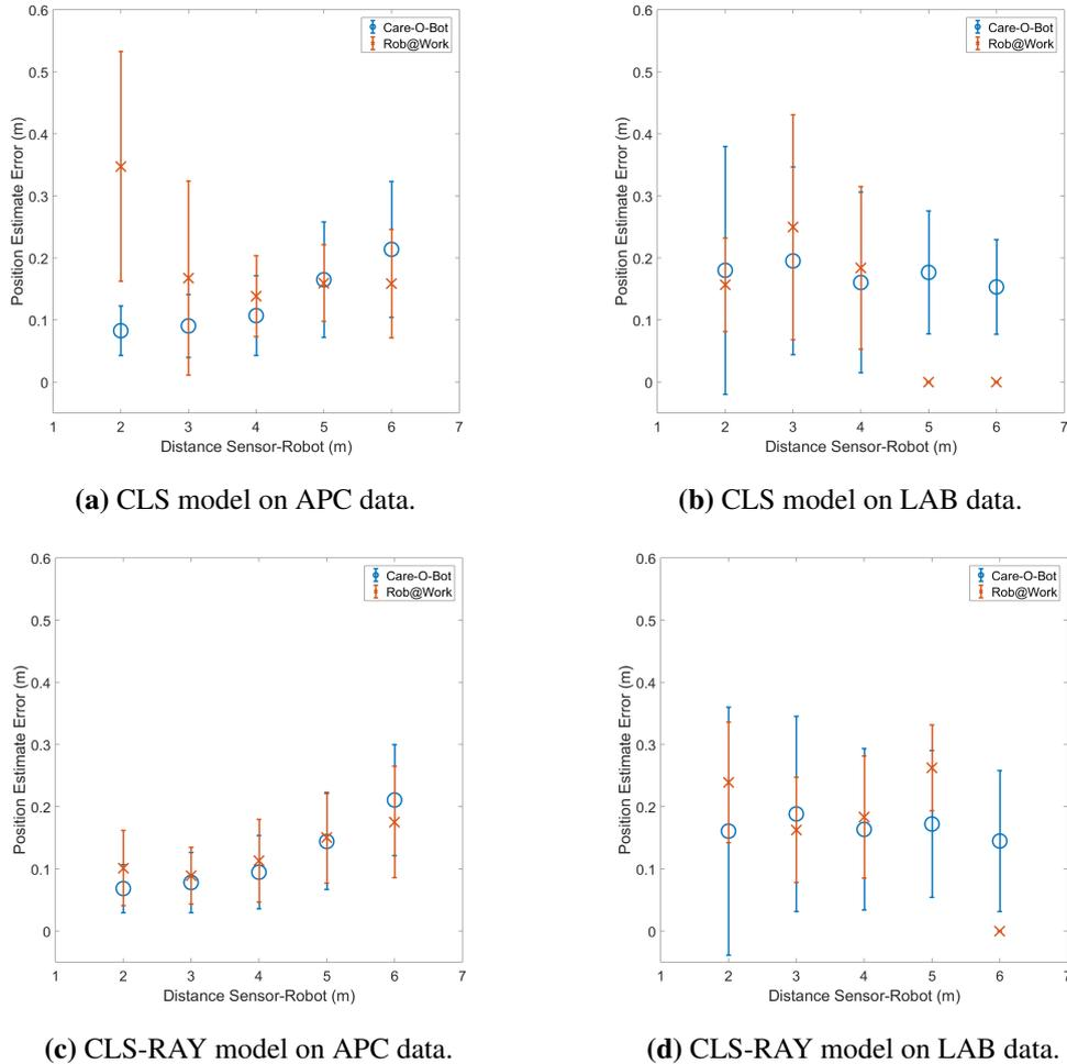
**Figure 6.5:** The mean error and standard deviation of the position estimation using the CLS/CLS-RAY CTD model on data-sets from the LAB and APC rooms. Each bar at  $x$  represents all position estimates between  $x - 1$  and  $x$ . There are no position estimates for  $x < 1$  because the size of their respective shapes prevents such close constellations.
