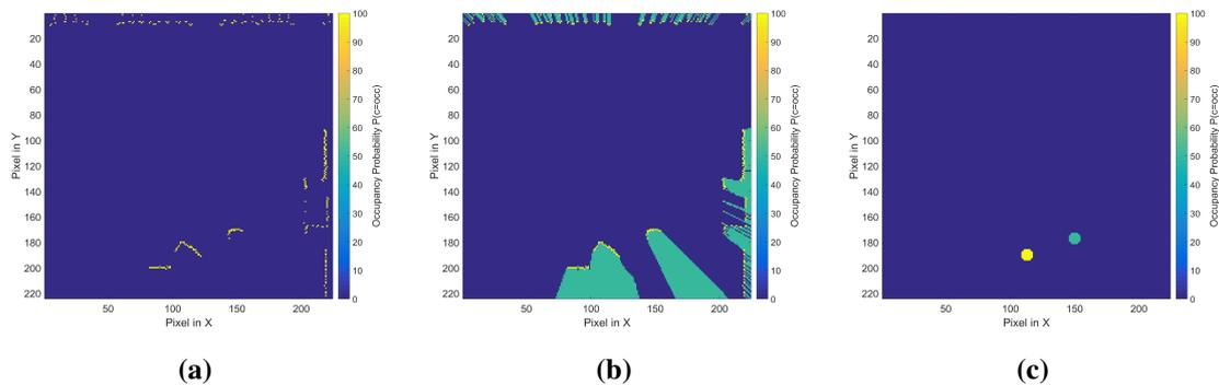
**Figure 5.3:** The in- and output of the classification networks. The input without marked unknown space (a). The input with marked unknown space (b). The output for both networks, where each colored spot marks the position of a robot and the blue colored space everything else.
