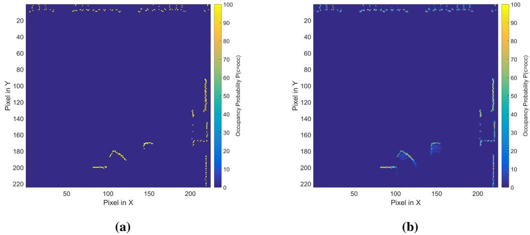
**Figure 4.5:** The grid-map generated from the laser scan for one time-step  $t$  (a). The color indicates whether the space (pixel) is occupied or free (blue). The same scene with accumulated data of the past 10 time-steps (b). The grid-map at the current time  $t$  is additionally multiplied with 10 to highlight it.
