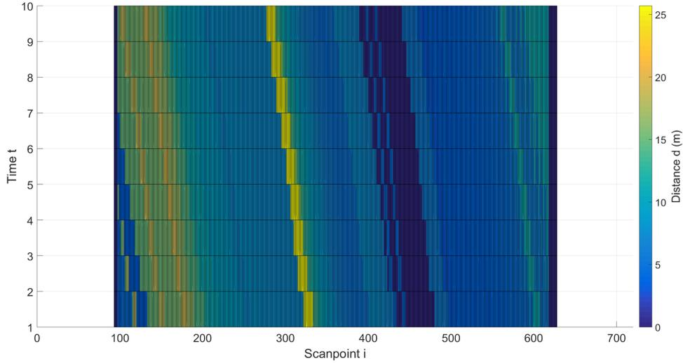
**Figure 4.3:** A plot of multiple (10) consecutive 2D LIDAR scans with each 541 scan points gathered from a sensor on a moving platform. The two light blue measurements around scan point 400 that continue to stay in the dark blue area throughout the 10 consecutive scans belong to a moving object. Due to the movement of the ego vehicle, the object can't be distinguished from the static background as in figure 4.2
