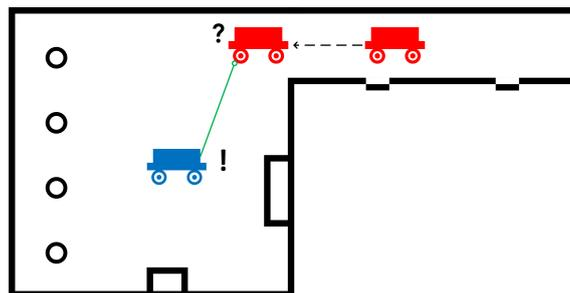
**Figure 1.1:** The problem, motivating this thesis. Robot A (red) is detected by robot B (blue), receives relative position information and improves its localization.
