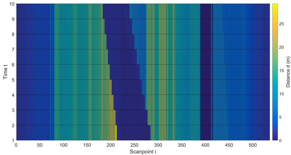
**Figure 4.2:** A plot of multiple (10) consecutive 2D LIDAR scans with each 541 scan points gathered from a static sensor. The blue measurements in the center around scan point 250 belong to a moving object. The changing location of the measured object form spatio-temporal features if stacked as in this example.
