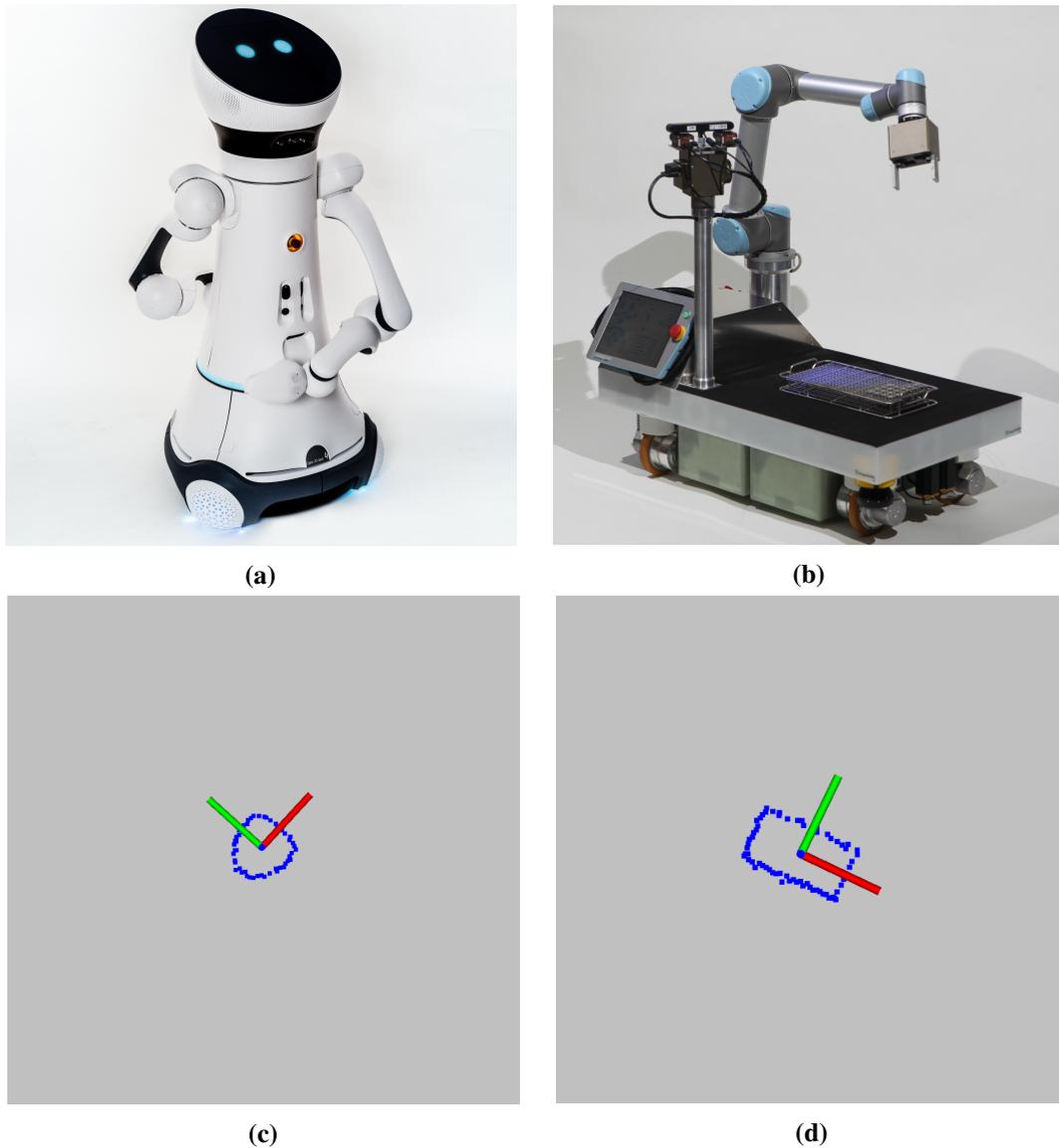
**Figure 6.1:** The two robots used for the evaluation. A Care-o-Bot with a semi-circular shape (a,c) and a Rob@Work with a rectangular shape (b,d).
