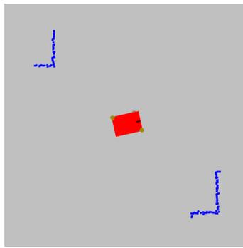
**Figure 5.2:** Two identically looking shapes detected by the 2D LIDAR. The shape in the top left corner is a rectangular shaped robot, while the one in the bottom right is an open corner of two arranged walls. Without the information about the sensor position, these two shapes are semantically identical.
