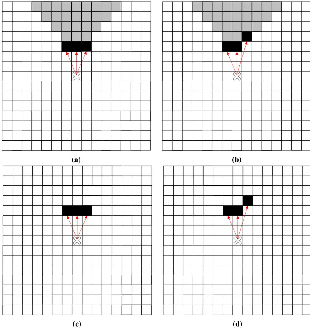
**Figure 6.4:** A scenario demonstrating the difference of the influence of a pixel-shift in the CLS-RAY data (a, b) compared to the CLS data (c, d). The images show the grid-map before (a, c) and after (b, d) the shift of the pixel.
