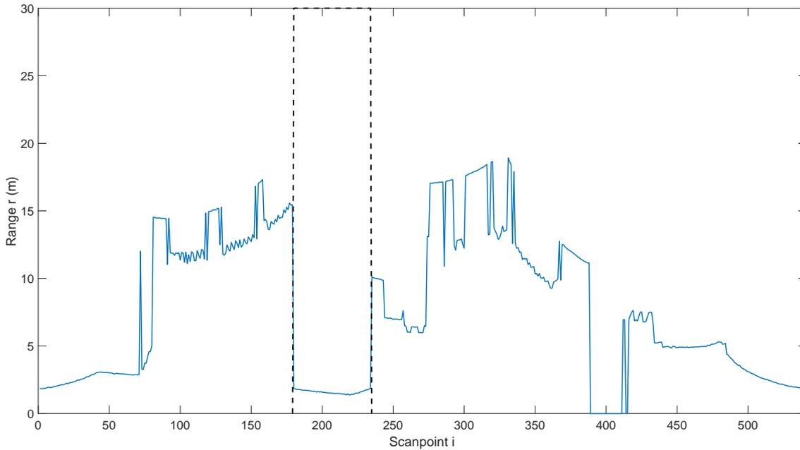
**Figure 4.1:** A plot of a 2D LIDAR scan with 541 scan points at one time step. The dotted line marks the scan points belonging to a dynamic object.
