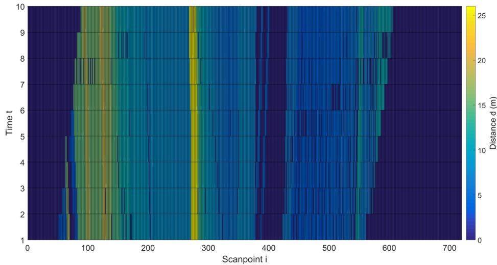
**Figure 4.4:** A plot of multiple (10) consecutive 2D LIDAR scans with each 541 scan points gathered from a sensor on a moving platform. All scans are transformed into the current frame ( $t = 10$ ). The scans are the same as in figure 4.3. The light-blue moving object is now easier to detect, since the surrounding background does not shift over time as much as in the non-transformed data.
