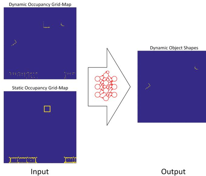
**Figure 4.6:** The input of the network using dynamic scan data together with a static grid-map is shown on the left. The right side displays the output of the same size where only the pixels belonging to dynamic objects are marked.
